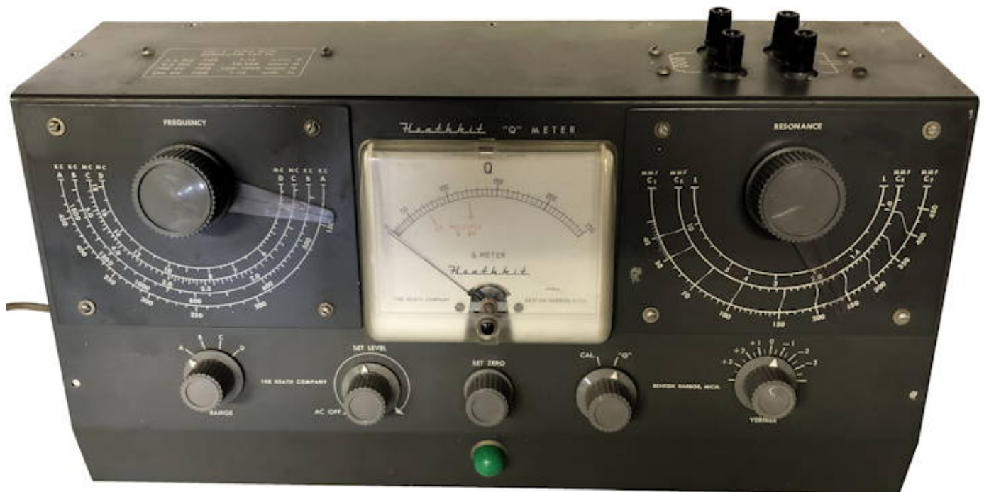
Figure 1: Front View of the Heathkit QM-1 'Q'-Meter. The unit is shown out of its cabinet.
